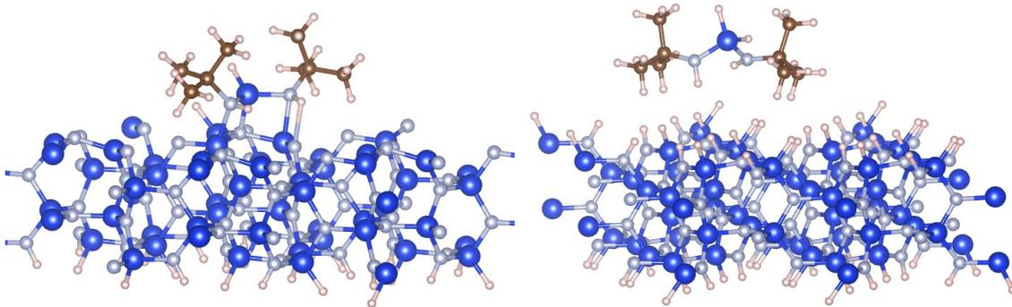
*BTBAS interacting with an under-coordinated bare  $\text{Si}_3\text{N}_4(0001)$  surface (left) and a H passivated  $\text{Si}_3\text{N}_4(0001)$  surface (right). While there is a strong interaction with the under-coordinated surface, the interaction with the passivated surface is very weak.*
