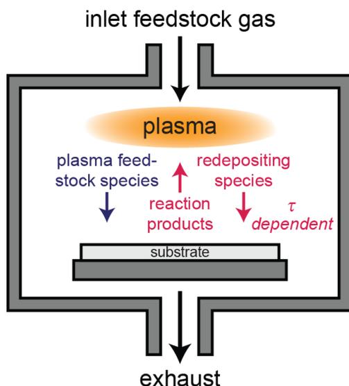
*Schematic illustration of general processes in plasma ALD. During the plasma exposure step, precursor ligands are liberated from the surface and enter the gas phase. These reaction products can dissociate in the plasma (e.g., by electron impact) leading to reactive species which can redeposit on the surface. The extent of the redeposition and its effect on the ALD process will depend on the gas residence time  $\tau$ , the used gasses, and the chemistry.*
