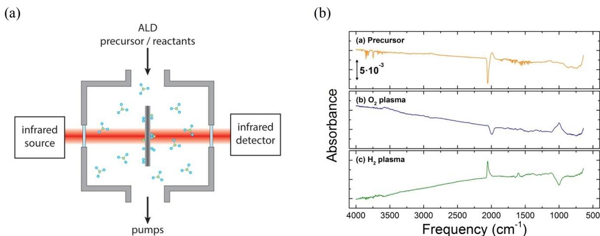
(a) Schematic representation of infrared measurements within an ALD reactor. Surface species and/or surface species can be measured. (b) Typical surface infrared spectra of the precursor, O<sub>2</sub> plasma and H<sub>2</sub> plasma step during the room temperature Pt ALD process.
