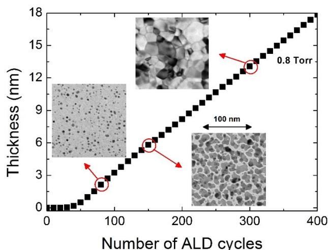
*Film thickness as a function of the number of cycles for Pt ALD on  $Al_2O_3$  as obtained by in situ spectroscopic ellipsometry data. The TEM images illustrate that Pt ALD evolves from island growth, via island coalescence, to film closure.*
